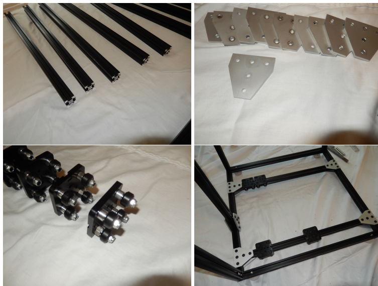
Figure 8: OpenBuilds Components. Upper Left: black anodized aluminum extrusion rails cut to length, Upper Right: plates for making T-joints, Lower Left: gentries, Lower Right: Partial assembly of coil winder.
